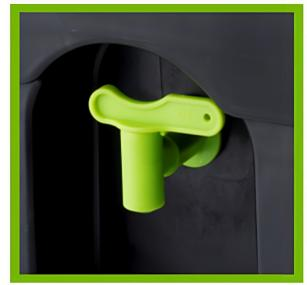
When installing the tap be careful not to strip the thread. When installing it secure the nut in place first and tighten it by turning the tap itself. If you get to a point where they are tight but the tap is not pointing in the correct position, loosen it off,
